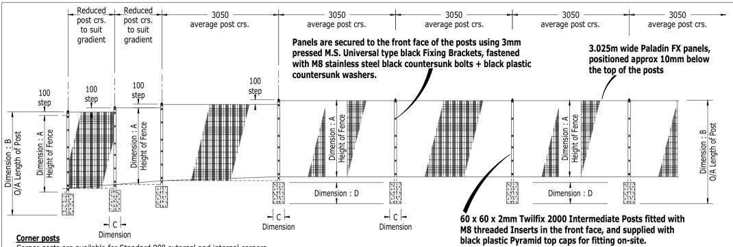
Corner posts are available for Standard 90° external and internal corners, and are also used for obtuse external and internal corners. End posts are not required.
